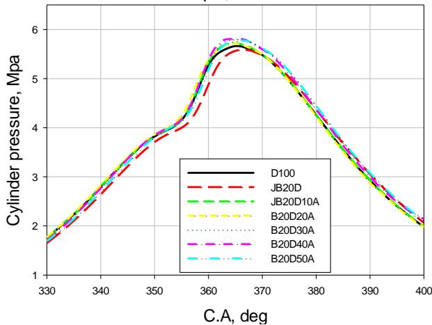
Figure 4 Variation of cylinder gas pressure with crank angle at 1500 RPM and 1300 RPM for 75% load
