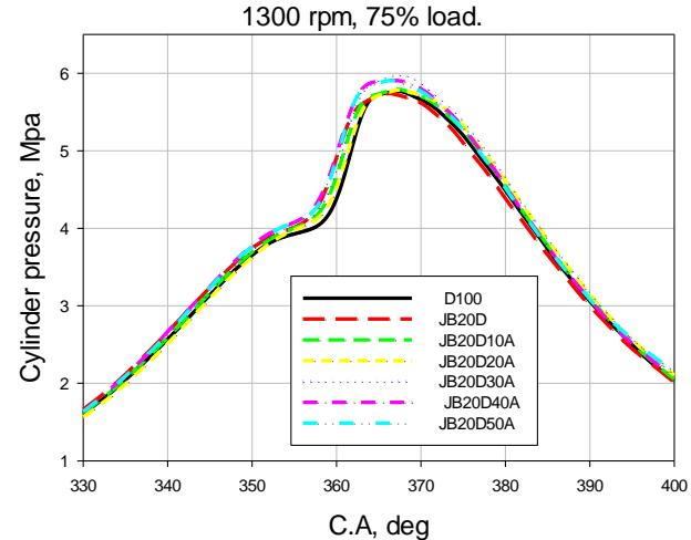
Table 7: The maximum pressure and its position for different tested fuels at 75% load for 1500 and 1300 RPM
