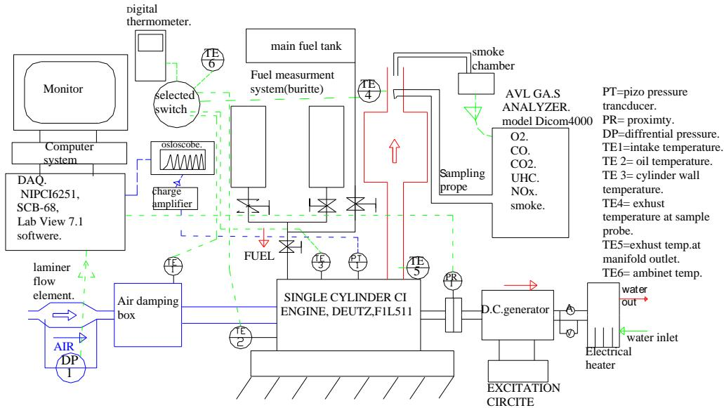
Figure 1: Schematic diagram of the test rig
