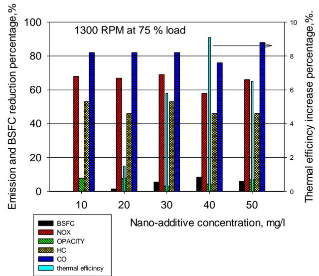
**Figure 10: The percentage change in engine performance indices as a function of nano dose in comparison with the corresponding values when biodiesel-diesel fuel is used; decrease of BSFC and NO<sub>x</sub>, HC, CO and smoke opacity emissions and increase of engine thermal efficiency**
