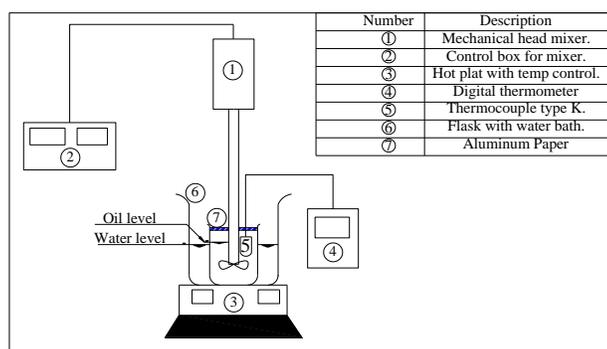
**Figure 2: Schematic diagram of JME preparation setup**
