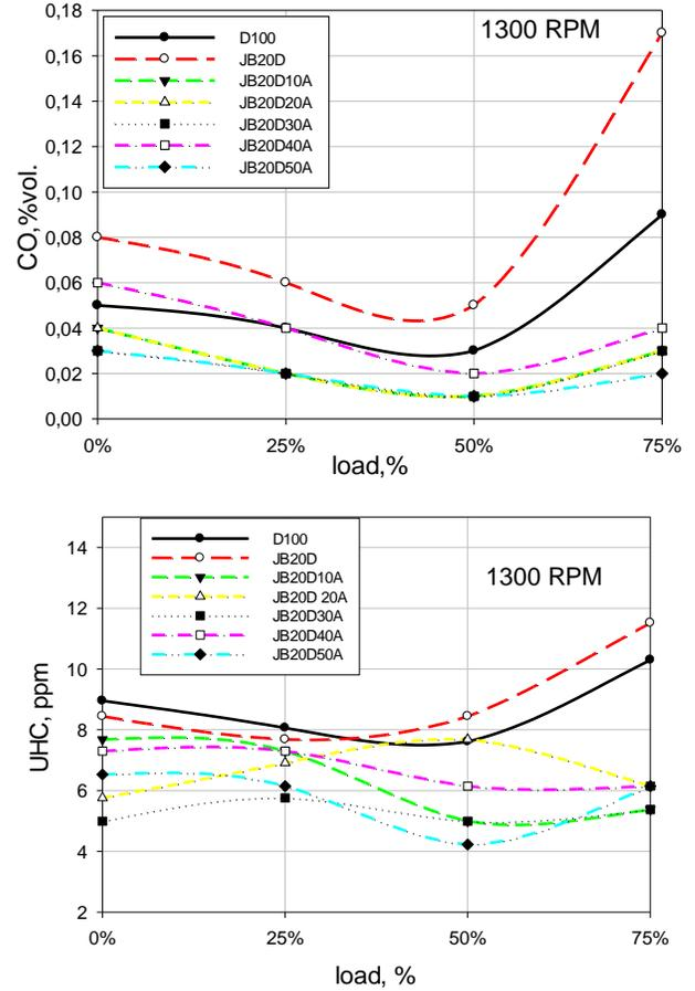
Figure 9: Variation UHC and CO emissions with engine load % at 1500 RPM and 1300 RPM
